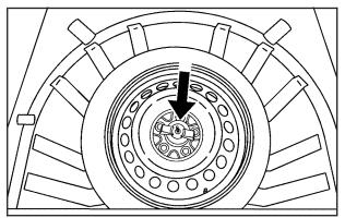
3. Turn the wing nut counterclockwise and remove it. Then remove the compact spare tire. See *Compact Spare Tire on page 381* for more information.
